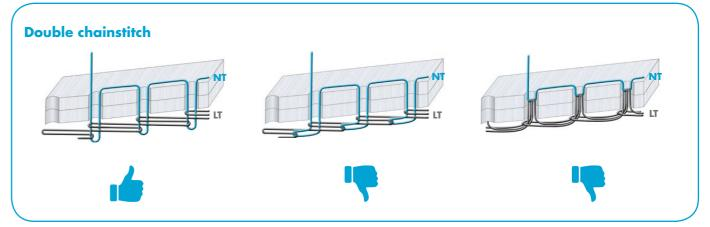
NT = needle thread | BT = bobbin thread | LT = looper thread
