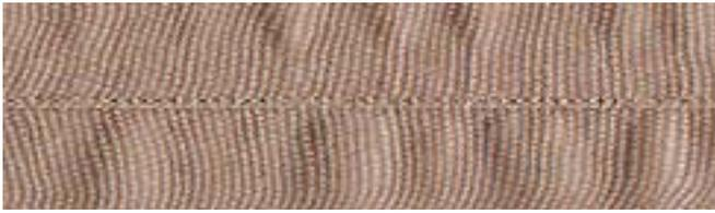
Identification: symmetric pucker at the left and right of the seam; pucker remains visible after thread is clipped between adjacent needle penetrations
