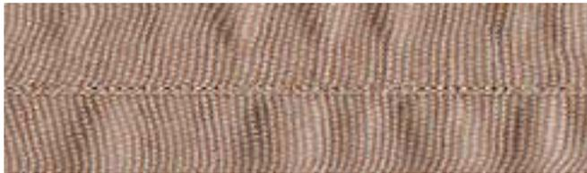
Identification: symmetric pucker to the left and right of the seam; pucker is gone after thread is clipped between adjacent needle penetrations
